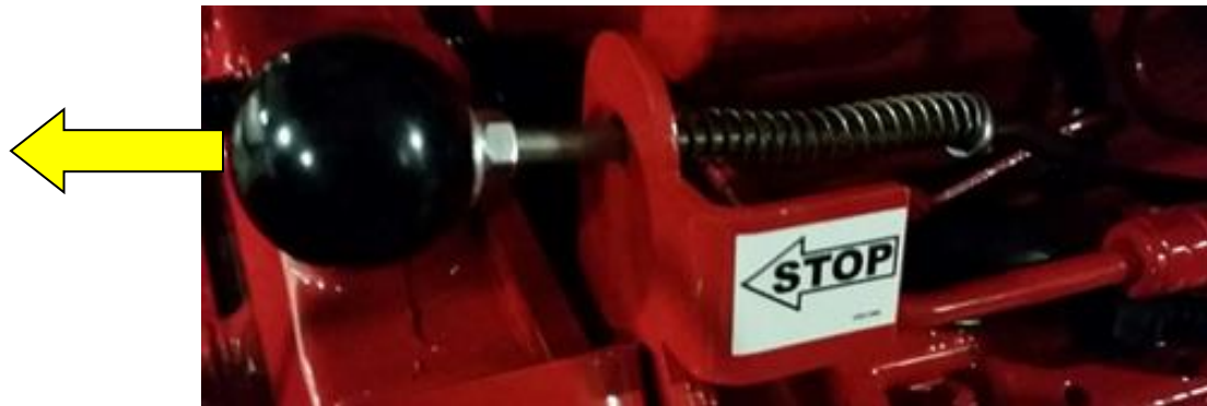
Figure 4b - JU4, JU6 manual stop override knob located on side opposite of instrument panel
