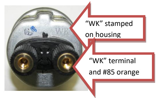
Figure 2b – JU4H, JU4R, JU6H, JU6R, KA4H, DP6H, DQ6H, DR8H, DS0H, DT2H, engine models: oil pressure switch – Jumper the "WK" terminal (orange #85 wire) to engine ground (battery negative)
