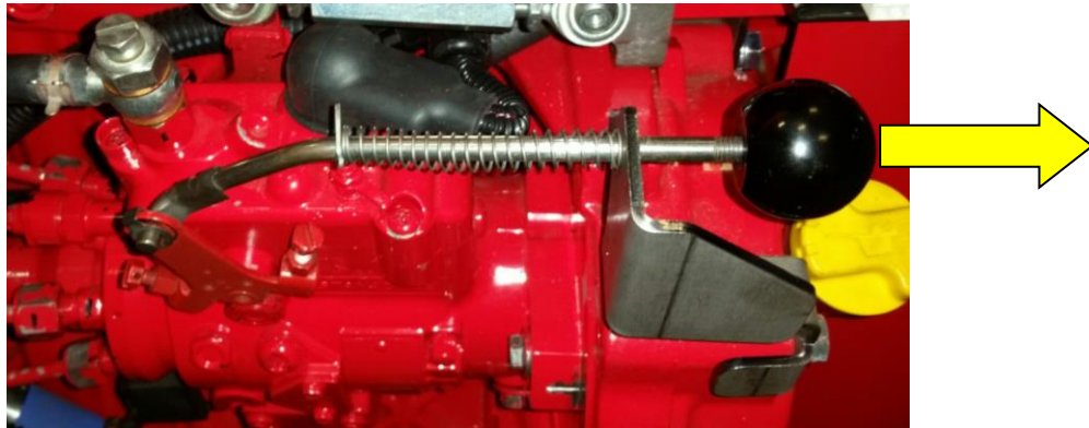
Figure 4a - KA4H manual stop override knob located on instrument panel side of engine
