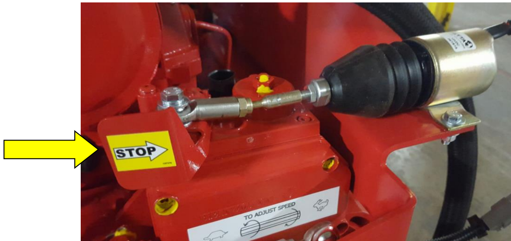
Figure 4d - ZE4H, ZF6H manual stop override lever located above flywheel housing
